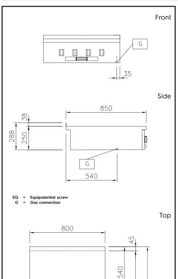
Gas Gas Power: 28 kW Gas Type Option: Gas Inlet: 1/2" **Key Information:** External dimensions, Width: 800 mm External dimensions, Depth: 850 mm External dimensions, Height: 250 mm Net weight: 65 kg Configuration: One-Side Operated;Top Front Burners Power: 7 - 7 kW **Back Burners Power:** 7 - 7 kW
